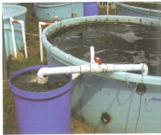
Figure 14.5: A settling chamber adjacent to a larger shrimp culture tank. Water is moved to the settling chamber using an air lift mechanism!
